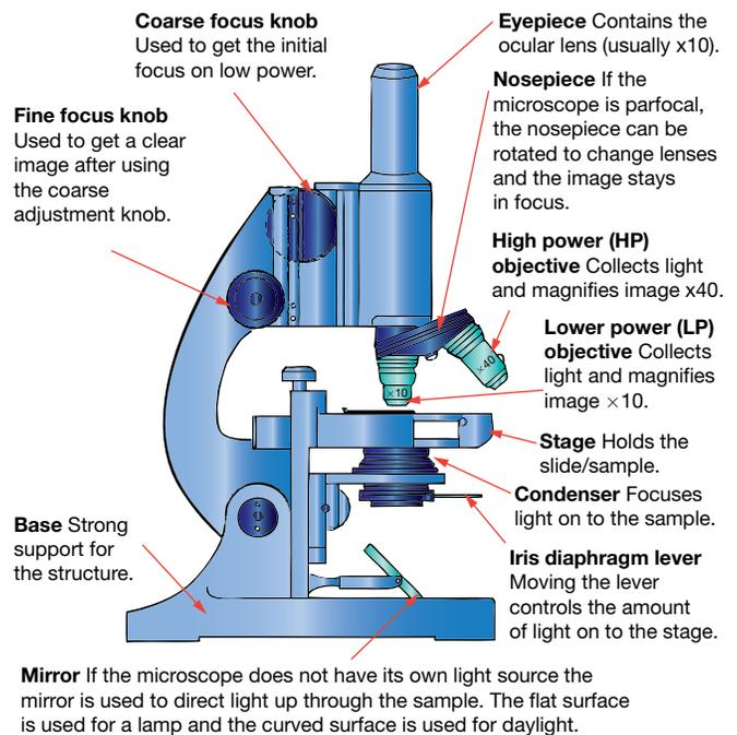
**Figure 4.2** Features of the modern light microscope.
