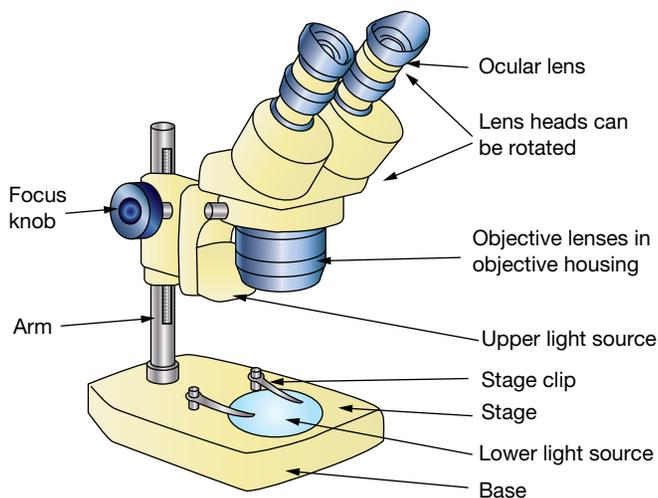
Figure 6.1 Stereo microscope.
